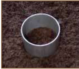
Figure 7.—Ring extends 2 inches above the surface.
