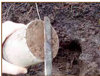
Figure 8.—Remove excess soil from bottom of ring.
